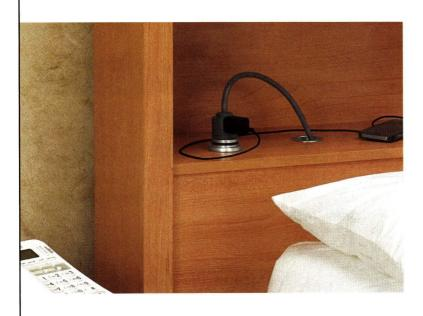
PCS56 provides pullout power when you need it and where you need it. Lift cap. Plug in. And go! Ultra convenient. Minimal footprint of 2" OD goes into 1 3/4" hole, 5/16" high. 13A, 125VAC, 7ft. cord. ETL listed, tested to meet UL 817. Finish: Satin Aluminum. U.S. Patent 8,475,186
