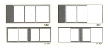
Multi-slide glass doors can be configured to stack to one side or two sides or can be designed to disappear into wall pockets.
