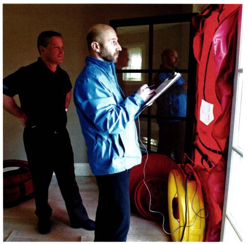
Blower door tests are the only satisfactory way to measure air tightness and highlight areas of heat loss.
