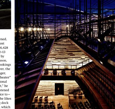
PERFECT CASTING The glass curtain wall on the performance hall's northwest facade creates an inviting 9,000-square-foot lobby (above), which doubles as a flexible performance space. The curved roof of the poured-in-place concrete structure follows the contours of the theater's fly space (opposite). A catwalk system above the audience chamber allows access to lighting equipment (left).
