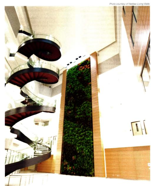
The five-story living wall at Drexel University's Papadakis Building in Philadelphia, designed by Diamond and Schmitt Architects and Nedlaw Living Walls Inc., is the largest of its kind in the U.S. With 1,500 plants integrated into the building's air handling, the system achieves an 80 percent air quality improvement and 30 percent reduction in energy consumption.
