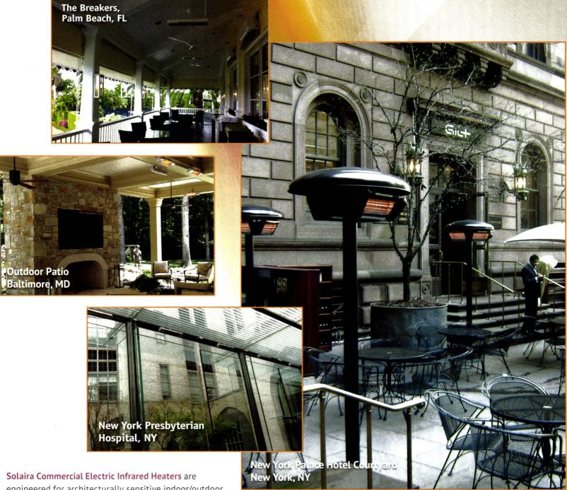
engineered for architecturally sensitive indoor/outdoor heating on patios, decks and waiting areas. Solaira technology converts 91% of the energy consumed into directional, comfort heating. Solaira Heaters achieve full output within 1 second and can also be controlled with digital variable controls, thermostatic, timer and occupancy sensors to minimize consumption.
