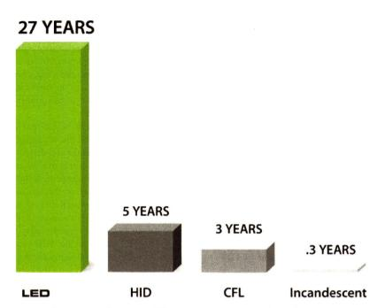
A comparison of the rated lifespan of different lamp types based on 10-hour-per-day operation.
