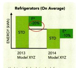
Updates to federal standards for refrigerators mean that in 2014 appliance manufacturers must effectively improve their models 20 to 30 percent over 2013 standards which are equal to or more efficient than 2013 ENERGY STAR® levels. To qualify for a 2014 ENERGY STAR® label, refrigerators will need to be 10 percent more efficient than the 2014 standards or 40 to 45 percent more than the 2013 federal standards.
