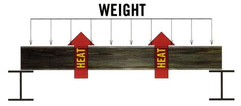
Steel has a small footprint, is non-combustible, and has excellent strength and structural properties. However, it has very poor thermal properties.
