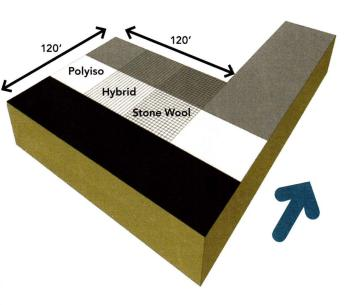
side-by-side roof insulation assemblies with variations in insulation make-up and roofing
