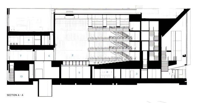
ACT I The theater (opposite) was designed for unamplified voices, so the architects worked with consultant Akustics to create the right distribution of reflective and absorptive surfaces. Matte-painted plywood boards of different widths are spaced two inches apart on top of fabric. "The wall panels couldn't be a sacred surface," explains David Haakenson, project architect, since set nieces could potentially be screwed into them.
