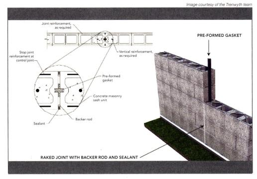
longitudinal movement, and separate dissimilar materials. Control joints, which are essentially vertical planes of weakness built into the wall to reduce restraint and allow longitudinal movement due to anticipated shrinkage, should be located where stress concentrations may occur. While these locations can be difficult to pinpoint in practice, following are some rules of thumb in locating the control joints. According to the National Concrete Masonry Association, these are:
