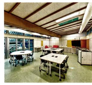
elements intended to promote student health and productivity such as architectural-grade storefront glazing, dimmable LED lighting controlled by daylight and occupancy sensors, and marker boards and tack surfaces as substitutes for typical finishes.
