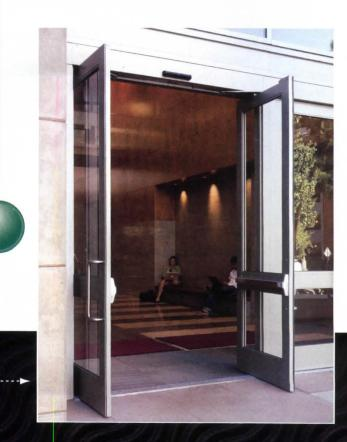
Power operation only when you need it. Balanced door operation when you don't. Our revolutionary design eliminates complicated, unsightly surface mounted hardware. A concealed low energy operator and actuating arm provide opening force on demand. Our standard hardware provides the closing force. When used manually PowerNow is pure Ellison.
