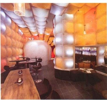
The grid of bubbles also perforates the facade to create a convex, pixelated surface. Additional glass pendants housing MR16 lamps graze seating areas, while downlights between the ceiling framework add ambient light.
