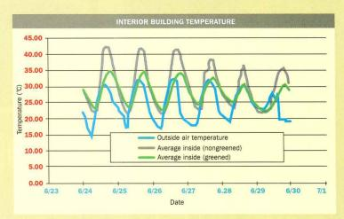
Penn State University Center for Green Roof Research A green roof can keep buildings cooler in summer (above) and can therefore help save on airconditioning costs, according to studies conducted at PSU's Center for Green Roof Research (right). This strategy makes most sense in regions with long cooling seasons.
