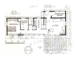
Floor plan, 1949 MIT solar test house, with an equipment room for the solar heating system about as large as the child's bedroom.
