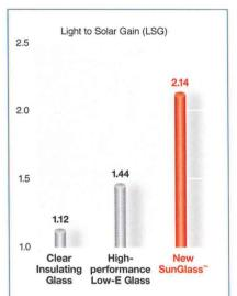
The Light to Solar Gain (LSG) value of solar glass far outperforms high
