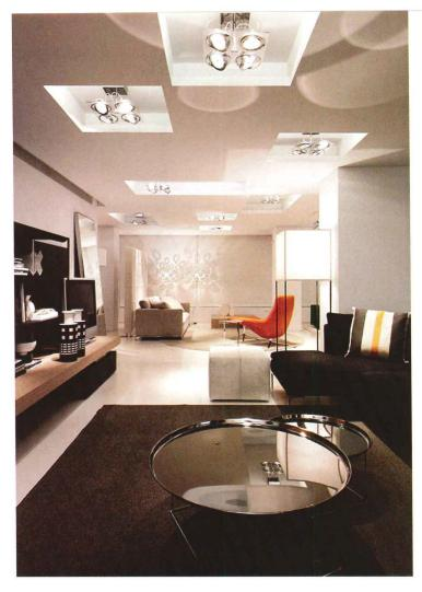
Throughout the showroom, Flos downlight units each feature four low-voltage lamps that can be tightly focused on furniture and accessories (above left and right). Illuminated with downlighting, a section of the wall beneath the staircase appears to float (below).
