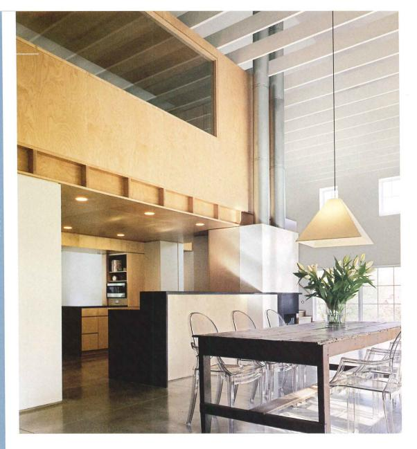
To preserve the loftlike space of the barn, the architects created an external buttress that allowed them to move the cross ties high up enough to get 16 feet of clear volume without beams. The kitchen is tucked under the upstairs bedroom, and the chimney flues thread through the cross ties to the rooftop.
