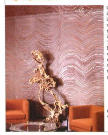
Gagecast® is a cast metal wall surfacing material suitable for a variety of interior architectural applications where patterns that feature high luster, relief, durability, and cost effective installation are a requirement. Twenty-eight designs are standard, however, custom collaboration is encouraged. Gagecast® is one component of Gage Vertical Surfacing. Contact the factory for product literature and selected samples. Email gage@centurytel.net
