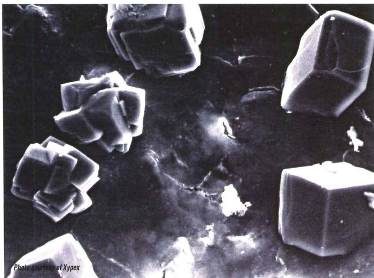
Scanning electron microscope (SEM) view of a concrete pore before the application of crystalline waterproofing.
