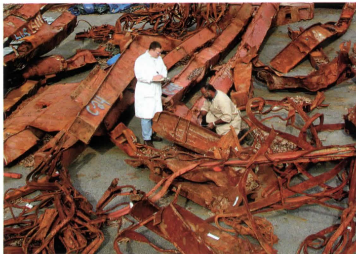
NIST research staff (left) inventory the steel recovered from the collapsed World Trade Center buildings (digital model below).
