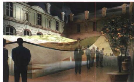
The gallery's curving roof will be made of glass disks.
