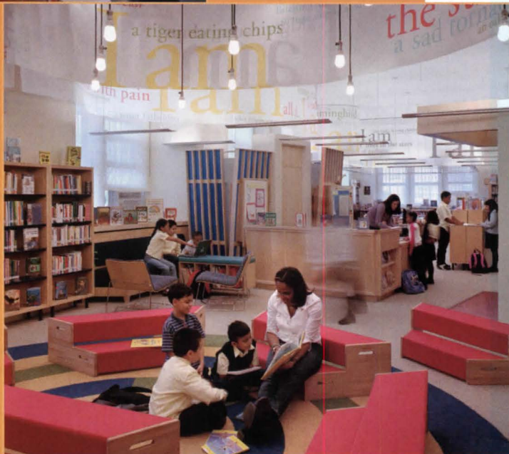
P.S. 192, Gluckman Mayner Architects From a ceiling, designed to look like a sky with clouds, suspended light fixtures resemble books with flapping wings. Bamboo floors, formaldehyde-free wheat-straw board for the casework, and recycled plastic are among the materials used for their low-cost and sustainable properties.
