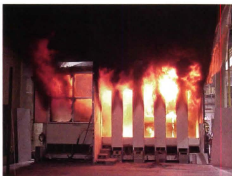
NIST conducted fire tests to assess the accuracy of computer models of the tower collapses.
