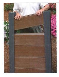
◄ Reduce noise and waste EverQuiet sound barrier wallboards from New Frontier Industries (NFI) typically reduce noise pollution by 50 percent. Manufactured from 95 percent postconsumer recycled plastic, the panels use a proprietary process that recycles a range of plastics beyond milk and soda bottles. The walls can be engineered up to 30' high and are capable of withstanding 150-mph winds. New Frontier Industries, Milton, N.H. www. newfrontierindustries.com CIRCLE 218
