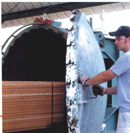
TimberSIL is a sodium-silicate-based pressure-treatment system for wood that relies on a mineralization process rather than toxins to prevent infestations and decay. Timber Treatment Technologies, Grosse Pointe Farms, Mich. www.timbersil.com CIRCLE 211
