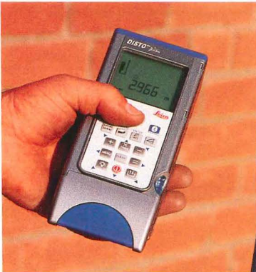
A handheld Leica DISTO and a PC with a Bluetooth device are all you need to create as-built drawings with PowerCAD SiteMaster.
