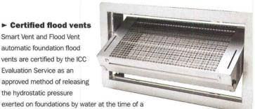
flood event. They open automatically, are bidirectional, and are manufactured of stainless steel to meet IRC and IBC building code requirements. One 8" x 16" vent protects 200 square feet of enclosed area below the base flood elevation. Smart Vent, Glassboro, N.J. www.smartvent.com CIRCLE 231
