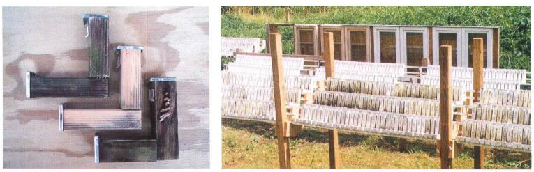
Left: Three unpainted L-joints in our greenhouse after 29 months exposure. The middle one is treated with the new process (machined from treated stock), with an untreated to the left (one of 3 of 10 that had not already failed), and on the right (fungus growing our) is a IPBC dip treated L-joint. Right: L-joints and window units in Hilo.
