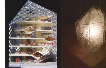
A model (above right) shows an early scheme to treat the building as a lamp with a double skin. Eventually, the architects took a different direction, in which a single skin is part of the building's structure. Horizontal tubes with dressing rooms inside (above) serve a structural role, as well. At night the finished building glows (right).
