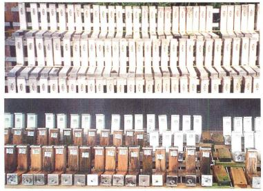
Top: L-joints during exposure in Hilo with differences in mold on paint. Bottom: Greenhouse setup of L-joints for artificial spraying of water.
