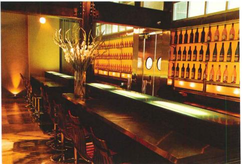
Vintage incandescent pendants and underwater halogens highlight the reflecting pool area (above). Linear fluorescents illuminate a bar top (left), with bottles backlit by PAR lamps fitted with yellow filters. Opposite, top to bottom: Zoned dining areas feature different colors of light. The restroom entry glows red beneath a chandelier. Boxes internally lit by incandescents punctuate pine-clad walls.
