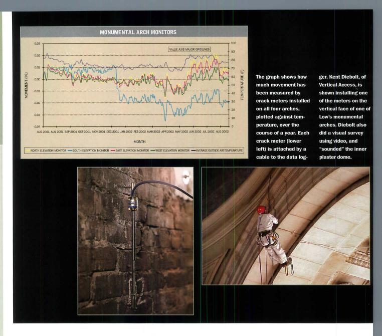
cracks did appear where the computer model led engineers to expect them: at the tops of the supporting arches. So far, there were no surprises. The last question was whether the cracks were getting worse.
