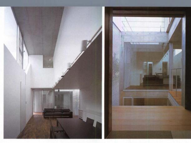
Because sleeping, living, and working all require a modicum of privacy, windows and direct outside exposure were kept to a minimum. Instead, daylight filters in through the glass walls at either end of the circulation zone, where there was no need for privacy since people go up and down stairs quickly. The ideal spot to open up to the outside world, these stairs double as a visual conduit linking the central courtyard and the side yards.
