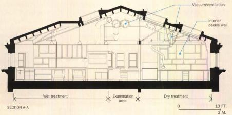
Custom workstations in the dry-treatment area (above) are spacious enough to accommodate both objects being examined and modern equipment. An interior wall (opposite) is composed of rectangular elements resembling deckles (paper-making frames); some pop out to display new papers.
