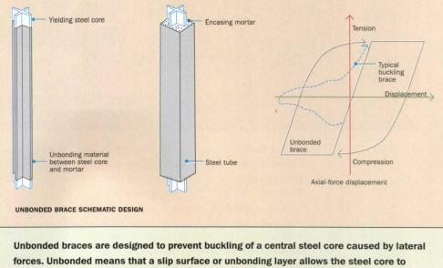
forces. Unbonded means that a slip surface or unbonding layer allows the steel core to move independently from the mortar and take all the axial loads.
