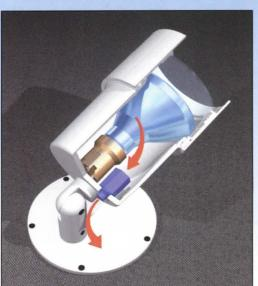
The ACV<sup>TM</sup> Valve System (Anti-Condensation Valve) utilized in B-K Lighting's PAR30/PAR38 fixtures expels moisture-laden air from the hermetically sealed optical compartment, creating an internal vacuum and eliminating the possibility of condensation. Leading industry organizations have awarded the ACV<sup>TM</sup> Valve System for it's unique and significant advancement to the art and science of lighting. Contact us today for more information.
