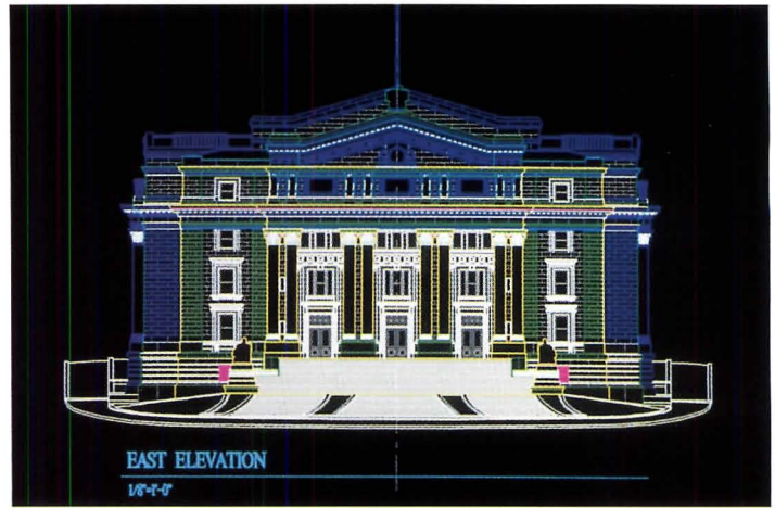
Ford Farewell Mills and Gatsch Architects scanned old drawings to create new digital images of the 1905 Essex County Courthouse in Newark, N.J.
