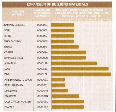
THE EXPANSION COEFFICIENT IS IN INCHES PER INCH PER DEGREE F. THE VALUE MAY VARY DEPENDING ON THE RANGE OF TEMPERATURE INVOLVED
