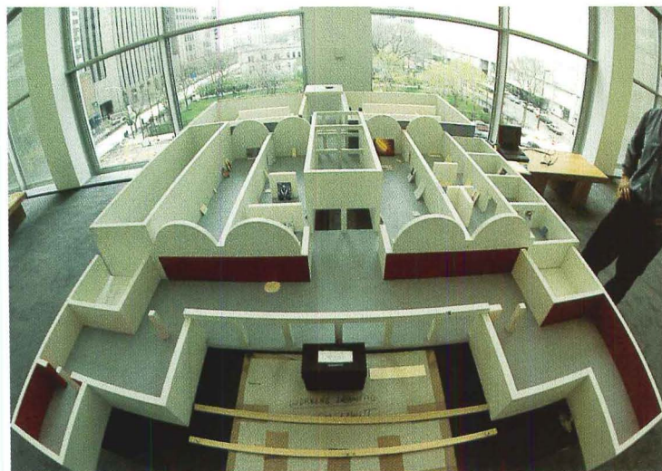
A model of one of the proposed MCA galleries (left). Rows of photometers are used to collect luminance data, and the video camera will be used to scan the model. The model itself (right) is very large.
