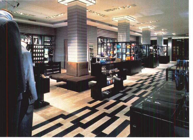
PAR 38 track lighting is recessed into light troughs, devised to help keep the ceiling free of clutter while providing plenty of positions for fixtures.
