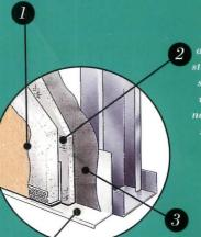
DUROCK™ cement panels are the most durable substrate in an exterior finish system. They won't trap water or vapor, delaminate, soften or deteriorate should water penetrate the system's exterior.
