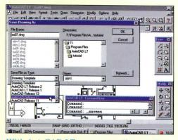
With AutoCAD LT, you can easily save R11 and R12 DWG formats with the command File Save As Menu. Note the floating command line window; it can be docked at the bottom of the screen.
