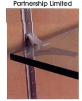
"ellen's brackets". an anodized-aluminum shelving system designed by M Ali Tayar. provides an elegant alternative to existing bracket-and-track systems. Cantilevered brackets come in two sizes, for shelves 3/4 or 3/8-in. thick and 10-in. deep. Wall-mounted tracks permit 1 1/2-in. adjustment of wood, glass or plexiglass shelves.
