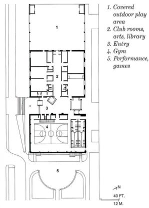
The architects transformed an unused ice-hockey rink into a new facility for the Boys and Girls Clubs of Boston, incorporating an outdoor pool into their design. Using existing foundations for the concrete-block gym, they inserted a new entry in place of two bays of the former rink. The rink's bowstring trusses cover new clubhouse facilities and, at the east end, a semi-enclosed play area.
