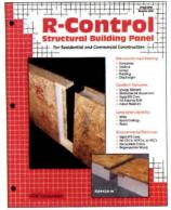
R-Control® Structural Building Panels provide superior insulation for walls and roofs in residential and commercial applications. EPS insulation is adhesively welded between stranded lumber facings, creating a panel that won't warp. R-Control has passed structural and fire tests as prescribed by national building code authorities. AFM's EPS contains no CFC's, HCFC's, or HFC's. R-Control, Panels are manufactured across the nation.
