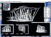
This model of the "Atlanta Pavillion," was modeled in form•Z and then used to derive plans and sections for construction documents.
