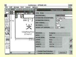
Plans and elevations in Abracadata are separate files. Object data in libraries can be very detailed.
