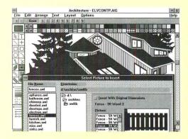
The foreground window shows the process for picking a fence from Abracadata's Architecture module symbols library. The drawing in the background is 2D, rendered in perspective.
