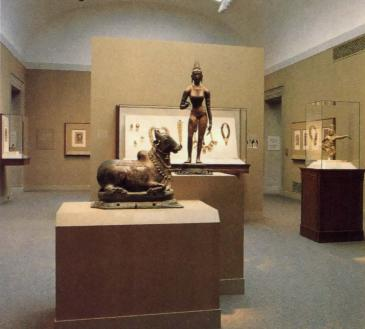
The walls in the Southeast Asia gallery (above) are very slightly washed with electric light to compensate for less light on cloudy days; a scrim behind the laylight protects light-sensitive artifacts. Focused spots and daylight pouring through a scrimless laylight constitute the illumination in one of the American painting galleries (opposite). The drawing (below) shows the relationship of skylight, scrim, and laylight.
