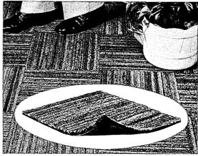
Exceptionally durable in heavy wear areas such as the entrances, lobbies and ramps of airports, theaters, factories and shopping centers. The carpet-like surface is made of heavy-duty tire stock, bonded to a flexible backing, installed with non-flammable adhesive and laid in a beautiful parquet pattern. Tiles are %" thick and 12" x 12" square. (Also golf spike resistant.)
