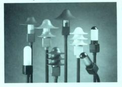
**320. Fluorescent landscape lighting** Scapeform fixtures use twin- and quad-tube compact-fluorescent lamps, with colorful (red, black, two greens, yellow, white) shades in several configurations. Most parts are made of molded polycarbonate described as virtually unbreakable. Line connections are made in the wiring compartment, so lights don't need a junction box or ground wire. W. F. Harris Lighting, Inc., Monroe, N. C.
