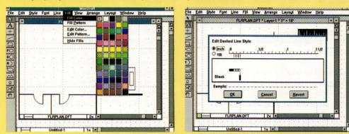
Selecting a fill pattern (left) on MacDraft with Windows. Notice that the fill color and pattern, and line type, appear at the lower left corner of any drawing window. When editing a line pattern (right), the pattern of dashes and dots will appear in a line as it is drawn.
