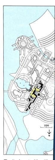
The site slopes to either side of the main axis that joins the en try roundabout with a knoll along the water. Another axis leads from the entry to the trapezoidal forecourt to Isozaki's building (future expansion is shown above).
