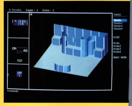
esignCAD's shading program allows up a eight light sources, but without choice of iffuse or point. Foregrounds can be ipped away. Four views can be displayed tonce (1, 2). Each view can be customized
