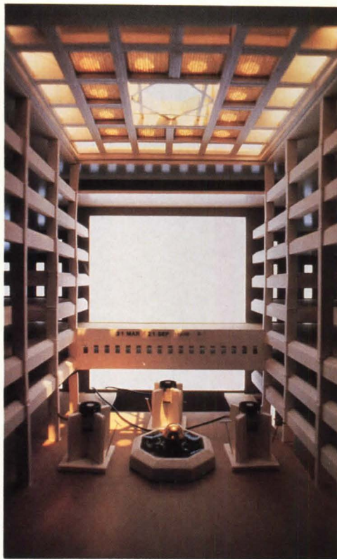
Sensors on the floor of the model measure the incoming light. In the background, an unobtrusive note labels the photograph so the designer can later compare conditions for a variety of times of the day and the year.
