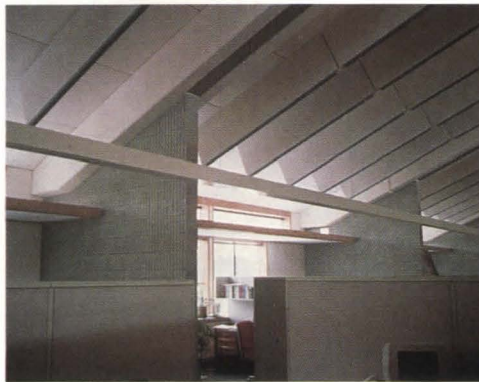
A relatively simple model (top) predicts light in the final building. Light shelves, paper blinds, and accurate surface colors distribute the light realistically. A mirrored side wall of a single bay represents the larger space.
