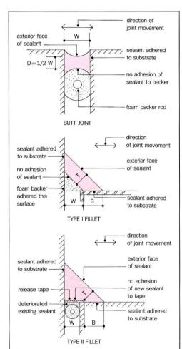
A typical butt joint (top). Two types of fillet joints and possible uses: at hollow metal frames (type I) and in remedial applications (type II).
