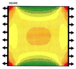
Computer-generated graphs indicate qualitative differences and locations of stress for various sealant configurations. Low stresses are blue to purple; medium stresses are green to yellow. Points of highest stress are red.
