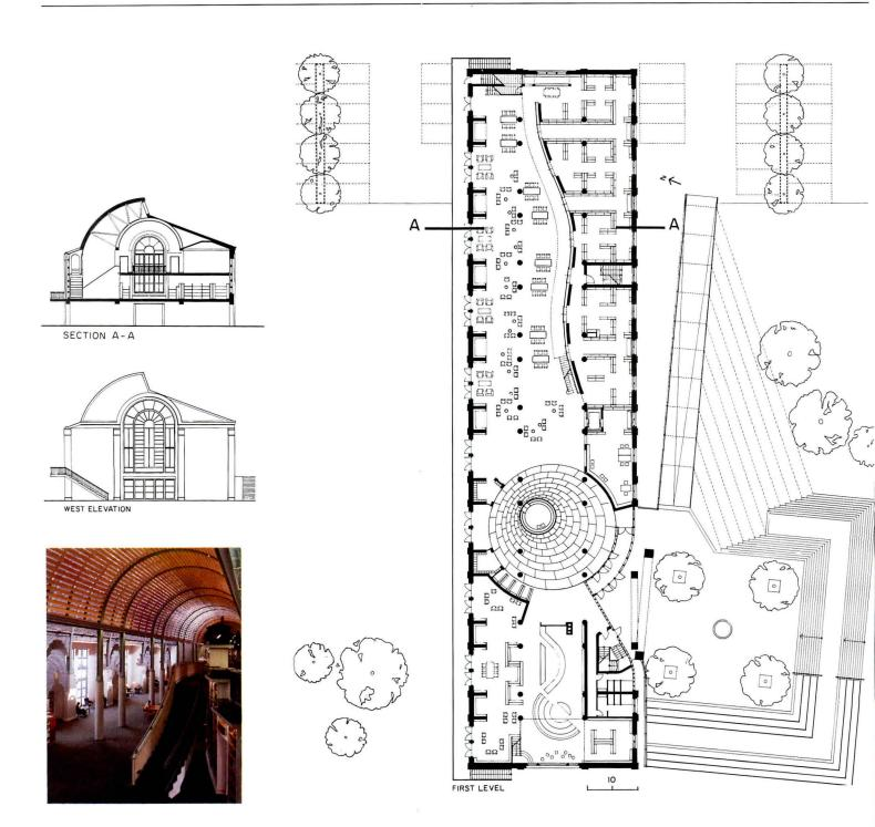
The library's steel and concrete frame is exposed on the interior. From the rotunda, a grand wall of books meanders along one side of the main reading room, and gives access to the open stacks and smaller reading alcoves beyond. The top tier of the doublelayered ceiling is sheathed in perforated corrugated aluminum. Lit by clerestory windows, it bounces light through the wood-slatted lower layer.
