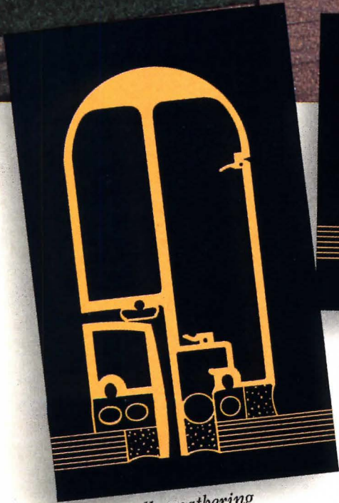
Sealair bulb weathering to reduce air infiltration at door perimeter.
