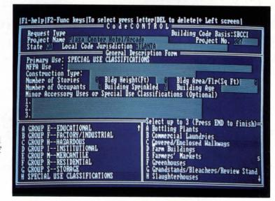
Data that describe the project are entered in the first screen (top). Among CodeCONTROL's helpful features is one that flags the selection of an inappropriate construction classification. The second dataentry screen lists code subjects that can be selected for further investigation (bottom). The subjects are nested for easy scanning; subcategories are revealed once a main subject is chosen. PLOT FASTER, LONGER, EASIER!
