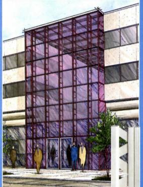
But while the design options offer flexibility, the integrity of the structure remains inflexible. A thermal break, and the flexibility of either 1/4" or 1" glass attest to Trusswall being ready and willing to take on nature's harshest elements.
