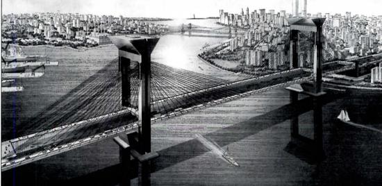
puble-decked steel-truss padways. One bridge will be instructed immediately south of e existing span, the other on e same location as the present idge, after its demolition. The chitects have designed parks, rusing, playgrounds, and other aces for public use at the proaches.
