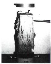
Fibermesh enhanced concrete column was compressed 10% of its original 21" length and still remained intact with very little spalling.
