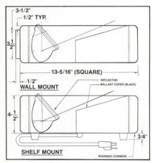
are four standard colors (with others available on special order). Construction is of extruded aluminum. The asymmetric reflector is adjustable. The ballast is integral. Two models are available: wall mounted (on a 1/2" reveal mounting plate) or shelf mounted (with cord, plug, and illuminated rocker switch).
