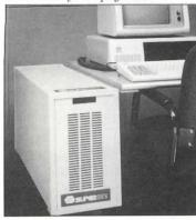
Graphics extension processor Current applications of the XP/48 graphics extension processor include two- and three-dimensional presentation graphics, solid modeling, computer animation, image processing, world mapping, and custom type-font generation.
