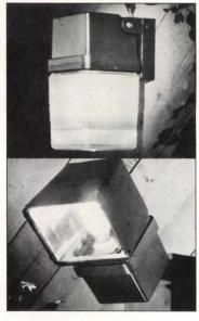
An area light and floodlight can be wall, ceiling, ground, or pole mounted. The area light is available in 35-, 50-, and 70-watt high pressure sodium and the floodlight is available in 35-, 50-, 70-, 100-, and 150-watt HPS. Both units are made of die-cast aluminum and feature a Duraplex II bronze finish. Stonco Lighting, Union, N. J. Write 391 on reader service card
