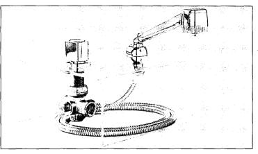
Shower system A deck-mounted shower system features a concealed hose, a fiveport diverter with 3/4-in. inlets for hot and cold water, a 3/4-in. outlet to the tub spout, and two 1/2-in.
