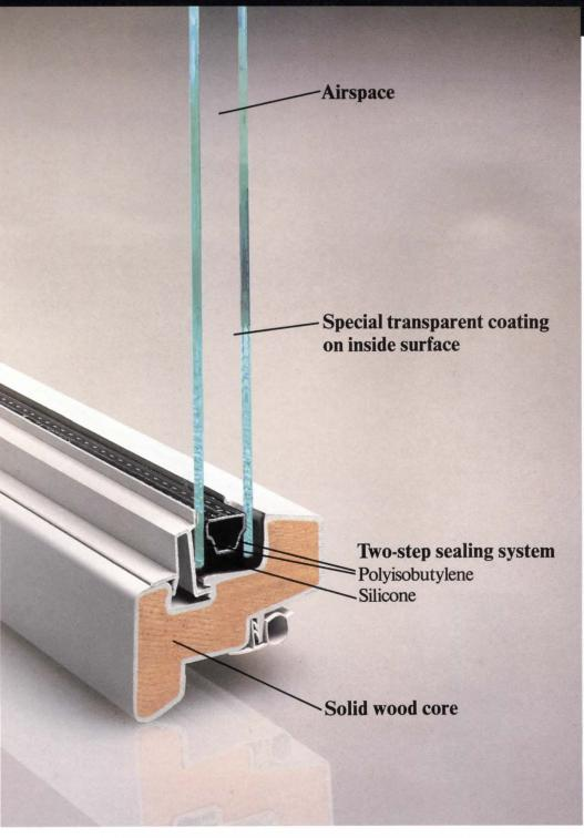
will appreciate that High-Performance glass filters out 71% of the sun's ultraviolet rays that cause fading.
