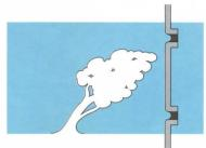
Tech Wall's patented and proven fastening system has been engineered to accommodate maximum thermal movement; condensation and weepage are controlled within the system.
