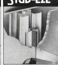
**STUD-EZE** is a flanged aluminum housing, with slotted heavy duty steel insert, designed to work with metal studs/dry wall application. Concealed slotting holds brackets for shelves, cornices, hangrail, etc.
