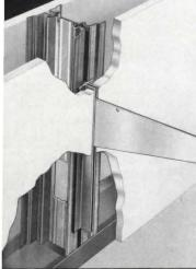
YOCA stud is a combination metal wall stud and slotted insert. Accepts dry wall and provides concealed slotted standards to hold brackets for shelves, cornices hangrail, etc. for stores, commercial and institutional construction.
