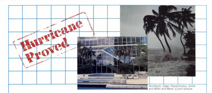
Past experience shows that windblown debris is a primary cause of glass breakage in a hurricane. Laminated safety glass effectively protects a building's interior from windblown debris. That is why it was specified for the first three floors of Ft. Lauderdale's new
