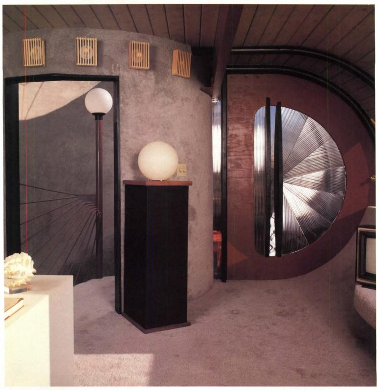
feet high at its apex and 40 feet in diameter, the studio is set into a windbreaking earth berm, much in the manner of Wright's 1945 Jacobs House. A corresponding circle, 30 feet in diameter, houses a kitchen/living room wing (plans overleaf). In both spaces 14-inch-wide poured concrete columns support a light-steel roof frame covered with translucent acrylic panels and tongue-and-groove wood siding.
