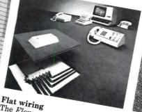
The Flexway undercarpet power system was designed to permit easy installation. It uses one tool and one connector for all taps, splices, and ground-shield connections. A protective bottom shield is adhered to the system's flat cable, cutting roll-out time. Burndy Corp., Norwalk, Conn. Circle 317 on reader service card
