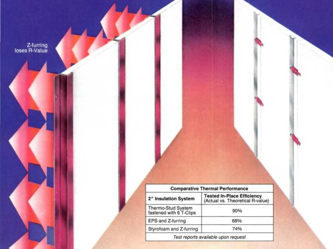
The one that fastens with Z-furring loses R-Value in a big way. Z-furring's metal channel conducts
