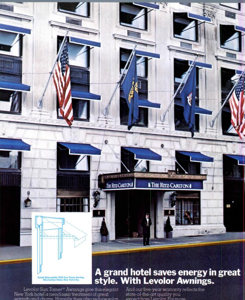
warmth and charm. Happily, they also reduce solar heat gain. Used systematically they can often reduce the size and cost of air conditioning equipment.
