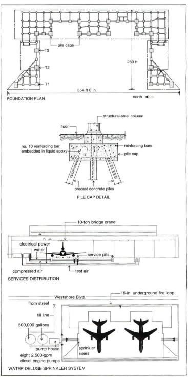
footprint while providing enough frictional force to neutralize the structure's susceptibility to wind uplift—because of its tremendous sail area. Of the 620 precast concrete foundation piles, 90 per cent were driven on a batter. The reinforced concrete pile caps to which columns are botted secure to the piles via hooked no. 10 reinforcing bars, which are embedded in the piles (see pile-cap
