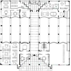
Although the neat symmetry was assisted by some fake (nonstructural) columns, the two furniture display areas flanking the central circulation spine are each three bays deep and three bays wide (plan above). Their north and south walls are conspicuously curvilinear to sustain Tigerman's fantasy: "I ripped the building apart, thus revealing the show room that had been there all along."
