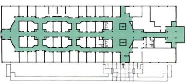
The spaces are heated and cooled according to a "thermal enclosure" concept. That is, the space within the over-all envelope is largely tempered with passive techniques, while a heat-pump mechanical system is directed toward the office enclosures within the envelope. To date, this design has yielded savings of approximately 27 per cent in heating and 21 per cent in cooling costs over a conventional system.
