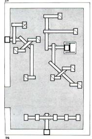
Photo 27: typical flat wire installation for power, telephone and data, Thomas & Betts; figure 28: computer-generated layout for power, telephone and data produced on a system comprising a Prime CPU, a Hewlett Packard 7580A pen plotter and modified Medusa software, AMP; figure 29: layout illustrating the principle of through-receptacle wiring and variable-angle cable bends, Thomas & Betts.
