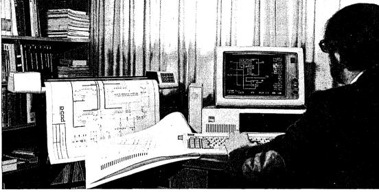
column plan, electrical distribution layout, duct layout, and lighting plan) on as many as 65 different layers, as though transparent overlays were used. Further, a symbol library of frequently used items, such as windows or desks, can be created and the symbols reused as needed. With a plotter or printer linked to the computer, a scaled drawing (or any portion of the
