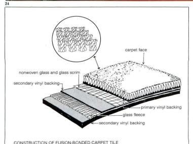
Photo 24: model P5300 Series fusion-bonded carpet tiles over flat telephone cable, installed at AMP Inc., Schaumburg, Illinois, Interface Flooring Systems; figure 25: construction of fusion-bonded carpet tile, Interface; photo 26: fusion-bonded carpet tiles, Milliken & Company.
