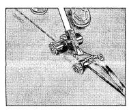
Roof membrane anchoring FasTrac is an anchoring system that does not penetrate its EPDM single-ply rubber membrane. A galvanized metal retainer track is screwed directly to the roof substrate. EPDM sheets are then laid over this track and a polymer insert strip is channeled into it to tuck and lock the sheets to the substrate. Firestone Industrial Products, Indianapolis.
