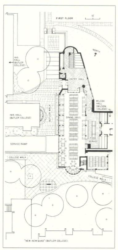
Venturi's ability to establish a balance between the formal and the casually disarrayed is evident in the plan. The building is not fixed in a particular relationship of configuration with any of its neighbors. It slides past 1915 Hall to the west and gestures strongly toward the "New-New Quad" to the south as it links the disparate existing parts of Butler College together. The dining hall sits as a
