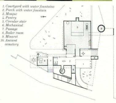
Ugljen placed the worship area and the courtyards with their ablution fountains (below right) beneath the levels of the market street and the surrounding cemetery, connecting these spaces to the sidewalk above by means of a curved ramp. This very subtle arrangement not only increases the sense of remoteness and privacy within the mosque proper but helps to insulate it against heat loss. The archetypical
