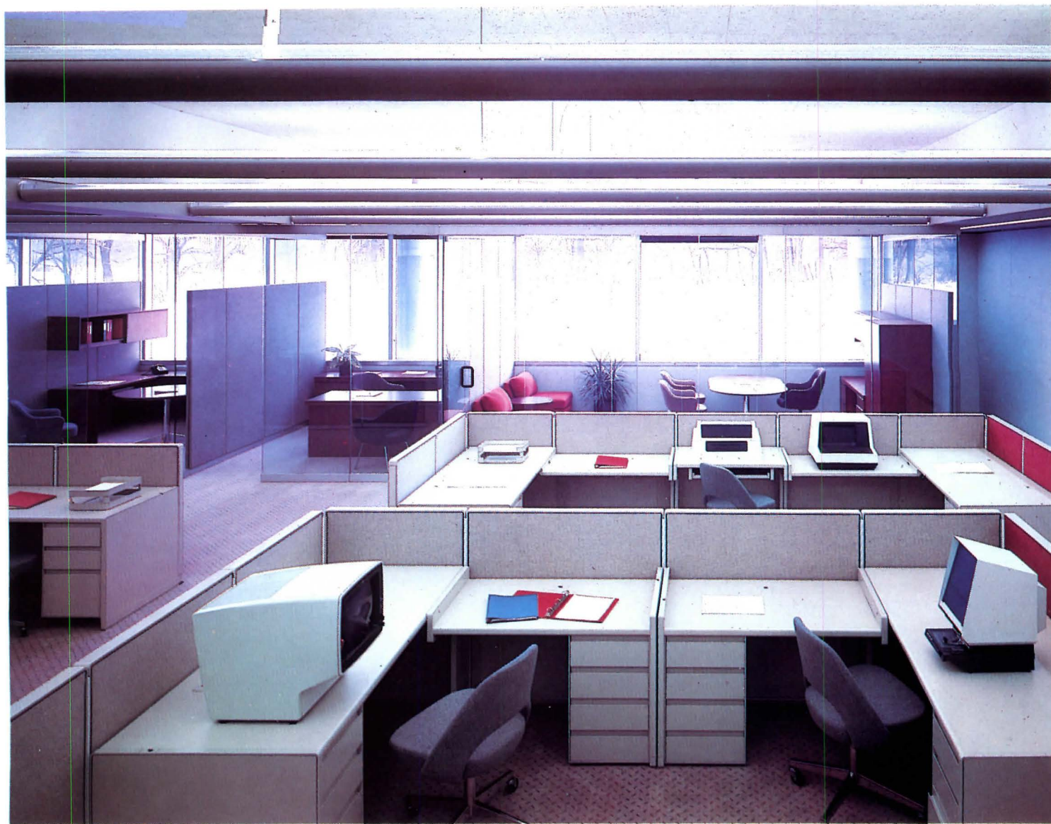
A view of one bay of the mock-up (above) shows the relationship of the transparent perimeter private offices to the interior work stations. The uplight reflected from the concealed-spline acoustic-tile ceiling has a pleasant, slightly-perceptible modulation which, with the transparent partitions, helps create the open feeling desired by the company. The 22-ft-long light tubes have one hanger in the center to control deflection. The indirect light from the tubes, fitted with cool-color, high-color-rendering lamps, complements the daylight from the windows. Evenness of the lighting has functional as well as esthetic attributes since it offers glare-free illumination for use of the CRTs. The system meets the Connecticut energy-code requirement of 1.6 watts per square foot. The outer three fixtures can be switched by a programmed light-control system.
