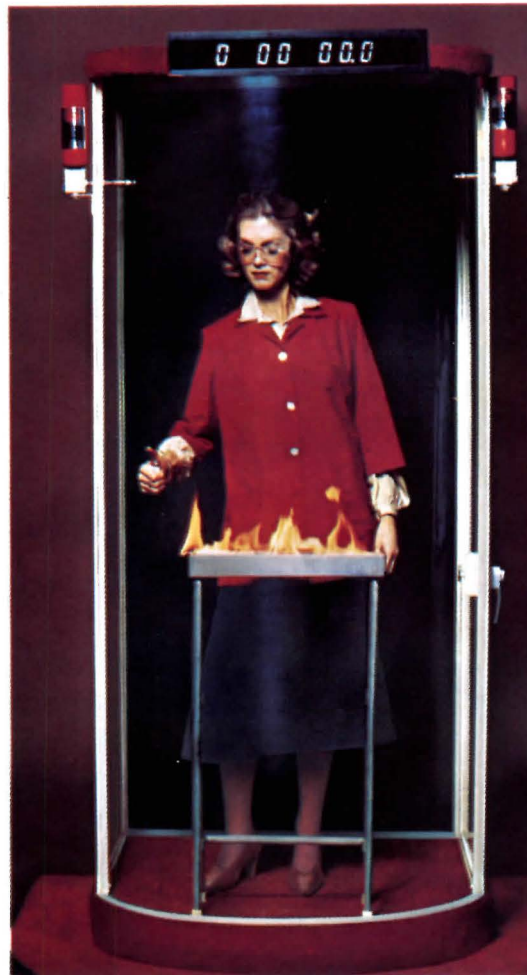
1. Flammable liquid ignited. Halon 1301 cylinders discharged.
