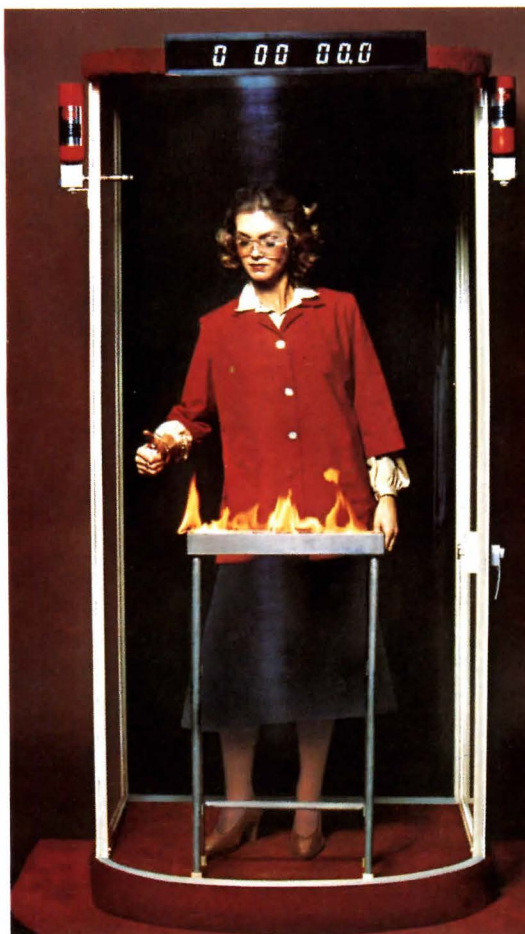
1. Flammable liquid ignited. Halon 1301 cylinders discharged.
