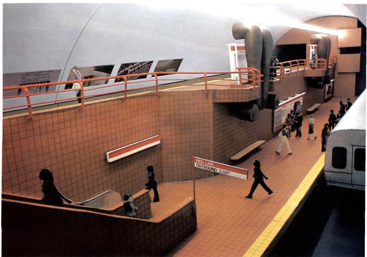
A glass headhouse is designed to pour as much daylight as possible into the subterranean depths of the deep-tunnel subway station at Porter Square in Cambridge. Passengers using the main entrance (top left) will descend to the large mezzanine (above), which also receives passengers coming from a headhouse across the street through an underpass beneath Massachusetts Avenue. After passing the turnstiles, subway riders immediately board super-long escalators to reach the trainroom 70 ft down (right). All riders cross a bridge to the upper platform, where riders going downtown catch inbound trains. Outbound riders take still another escalator to the lower platform.
