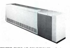
**REVERSE-CYCLE AIR CONDITIONER** / Engineered especially for school heating and cooling requirements, the EnerVent unit ventilator is a flexible system. The air conditioner absorbs heat contained in the winter outside air, adds heat from the compressor, and pumps it into the school room. The EnerVent uses outdoor air for ventilation cooling on moderate days. • American Air Filter Co., Inc., Louisville, Ky. circle 317 on inquiry card
