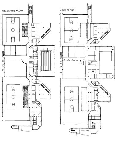
The main entrance from grade is shown in the photo at top. The building can also be entered by a pedestrian bridge at the mezzanine floor level where the main circulation spine is located. This spine is open to the double-height spaces (left in plan) and allows access to ancillary spaces on the other side.
