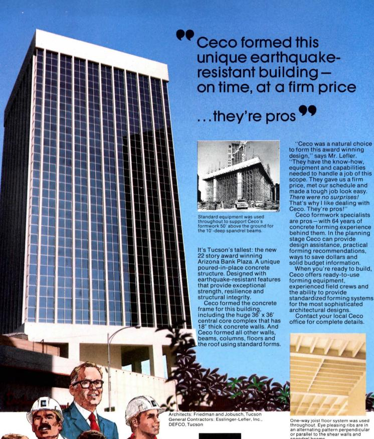
One-way joist floor system was used throughout. Eye pleasing ribs are in an alternating pattern perpendicular or parallel to the shear walls and spandrel beams.
