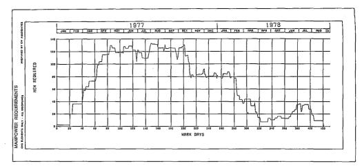
Figures 4 and 5. Based on production schedules and known requirements, CM Associates, Inc. uses a simple computer to forecast manpower requirements over approximately two years. The computer then charts this information, giving a quick view of
